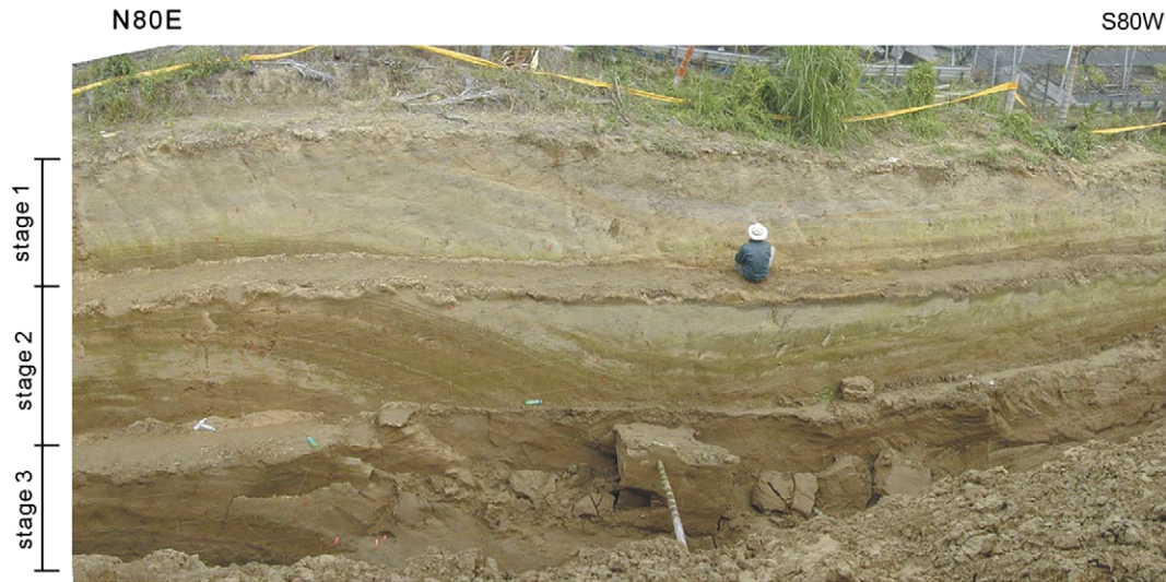
Fig. 1. Appearances of northern wall of the studied trench. The photo has been flipped horizontally for comparison with the inversion results. The trench has a length of 27 m and a depth of 7 m, which comprises 3 stages with a height of about 2 m for each stage. The monoclinical morphological features of ground surface and beddings, downward steepening of forelimb strata, and smoothly rounded fold-hinges are consistent with a trishear fault-propagation fold growing above a blind thrust.
